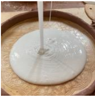
Figure 17 Negative silicone rubber mold
