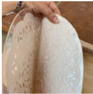
Figure 18 Silicone rubber mold
