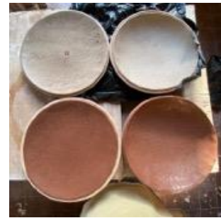
Figure 13 Pressed slabs on curved support
