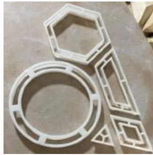
Figure 23 3D printed ring foot cutter
