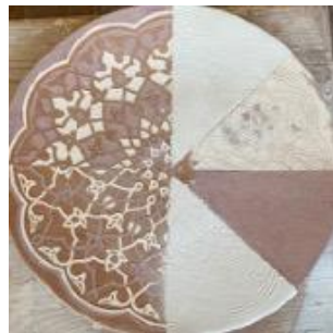
Figure 15 Slip & glaze samples on red clay
