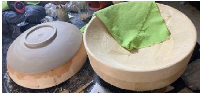
Figure 24 Negative & positive wooden molds
